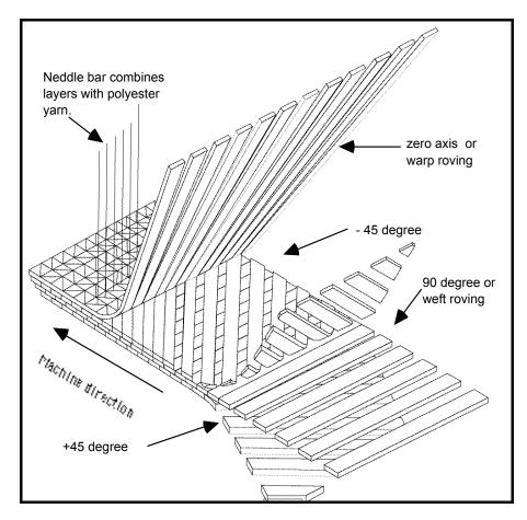
**Figure 1.** Stitch Bonded Example – Quadraxial<sup>1</sup>. Typical quadraxial ply stack. The 45° and 90° plies are interchangeable with the 0° always on top. Quadraxial fabrics can be made with equal weight in each ply, 0°, - 45°, 90°, + 45°, to produce a laminate of quasi-isotropic strength or unbalanced architecture to provide efficient support for rectangular panels.<sup>2</sup>
