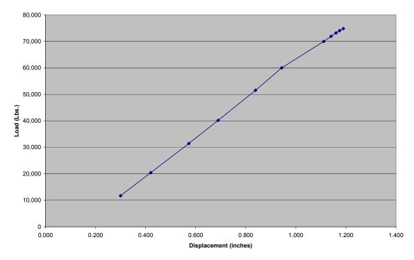
Figure 8. Plot of Load Versus Displacement for the 5" Deck Specimen. Single tube only.
