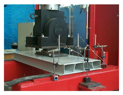
Figure 7. Static 3-Point Bending Test at CFL (NCSU) for the 5" Deck Profile; May 2001.
