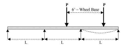
Figure 6. MMC's Definition of Stiffness for Decks on Bridges.
