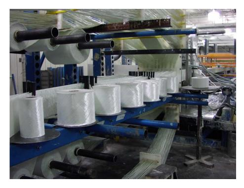
Figure 4. Fabrics and Unidirectional Fibers Being Pulled Into the Mold.
