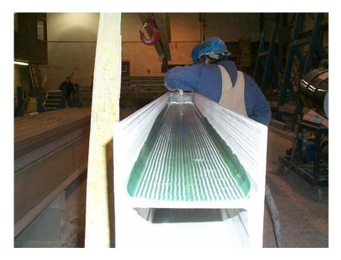
Figure 10. Adhesive Being Applied to the Female Part of the Bond Line Joint in the 5" Deck.
